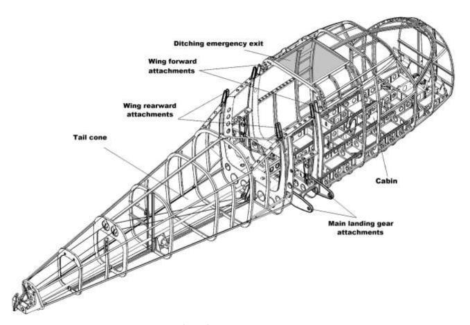
Figure 2. – Fuselage structure
