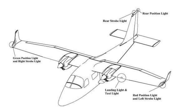
Figure 10. – External lights arrangement
