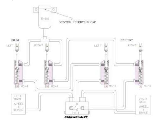
Figure 14. Brake system schematic
