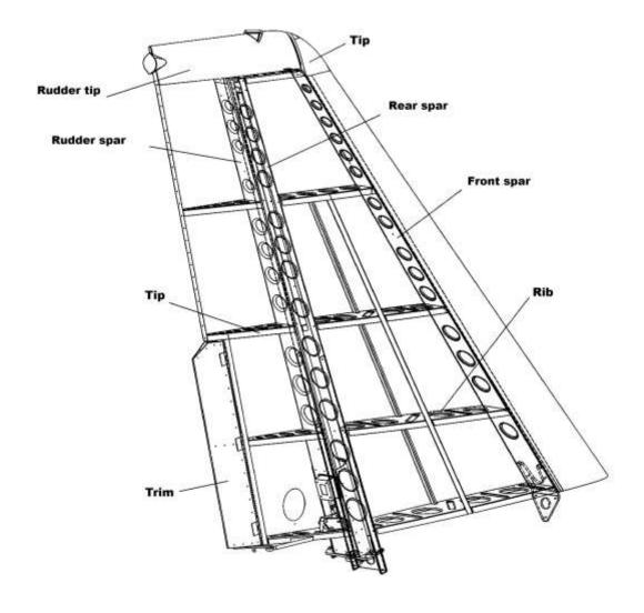
Figure 3. – Vertical empennage structure
