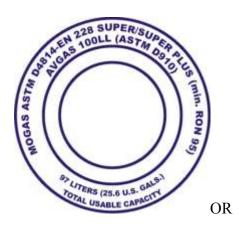
MOGAS ASTM D4814-EN 228 **SUPER/SUPER PLUS (min. RON 95)** AVGAS 100LL (ASTM D910)
