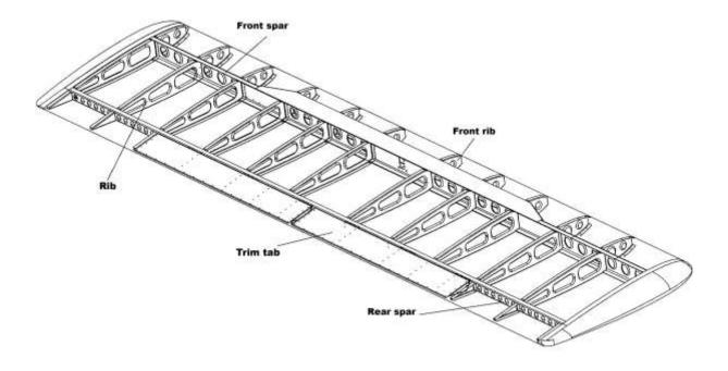
Figure 4. – Stabilator structure
