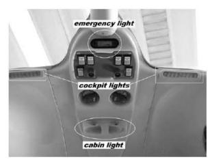
Figure 9. - Over-head panel lights arrangement
