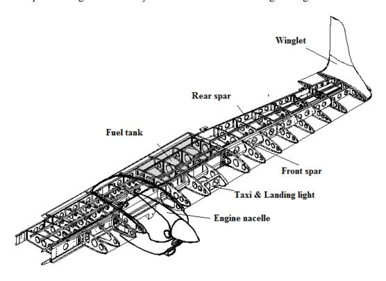
Figure 1. – Left wing structure
