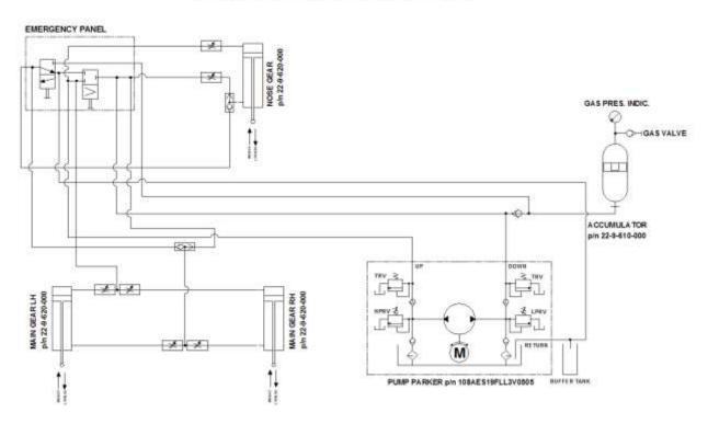
Figure 13. LG hydraulic system schematic
