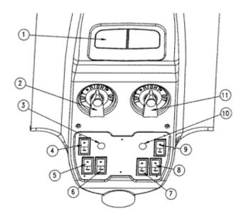
Figure 8. – Cabin head panel controls
